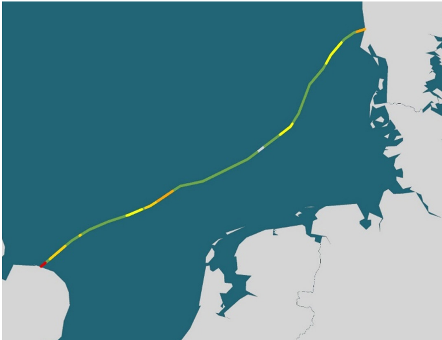
Figure 5: An example fault prediction map for a fiction cable system across the North Sea
