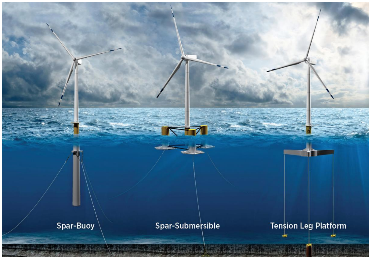
Figure 6: Offshore wind floating foundation concepts
